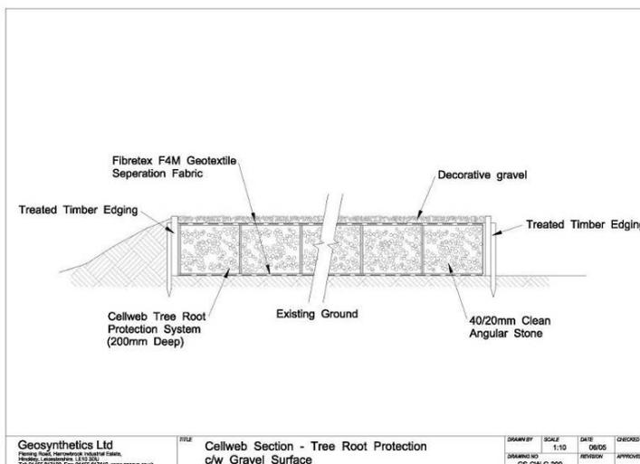
This image shows a proprietary brand of “Cellular Confinement” system that will provide load bearing capacity for vehicular passage whilst preserving the ground environment beneath the system.
