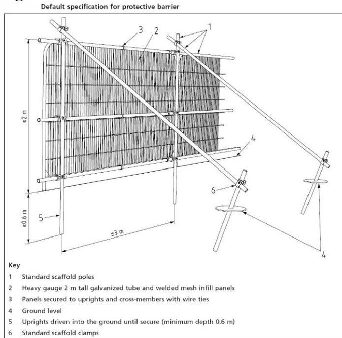
This image illustrates one possible option for the construction of the “Construction Exclusion Zone” protective fencing.
