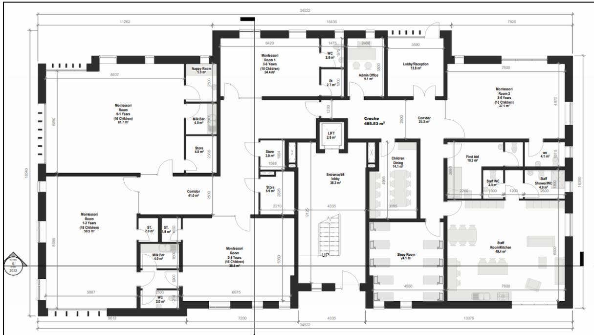
Figure 4.0 Proposed ground floor level of Block F illustrating layout of creche facility.
