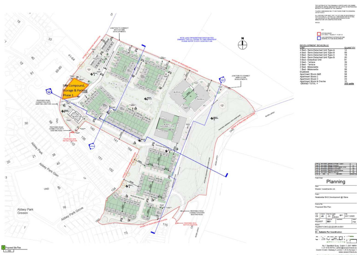
Figure 3 – Site Compound, Parking & Storage Location
