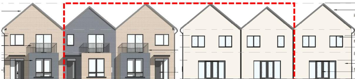
Figure 80.0 Front elevation of House Type 5.1 (left) and rear elevation of House Type 5.1 (right). The area within the red dashed lines represents the front and rear elevations of House Types 5.2 & 5.5.
