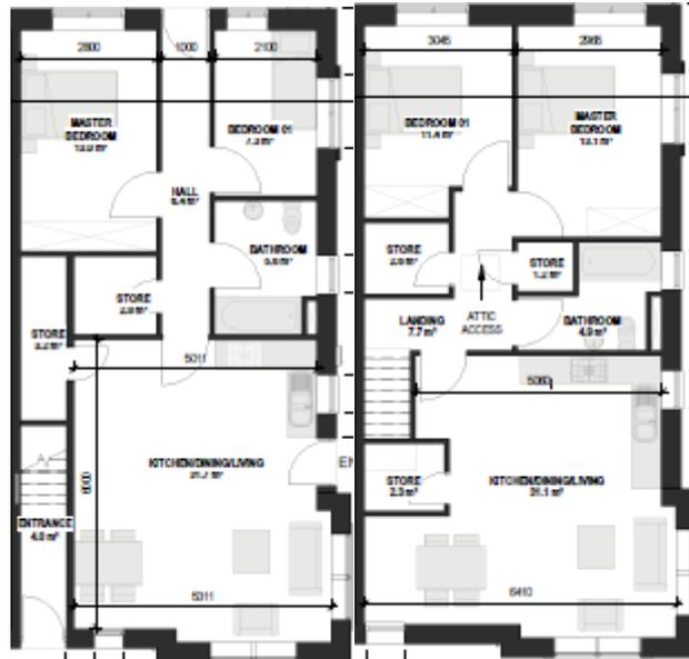
Figure 42.0 Floor plan of Maisonette Type 7.5 (left) and floor plan of Maisonette Type 7.6 (right).
