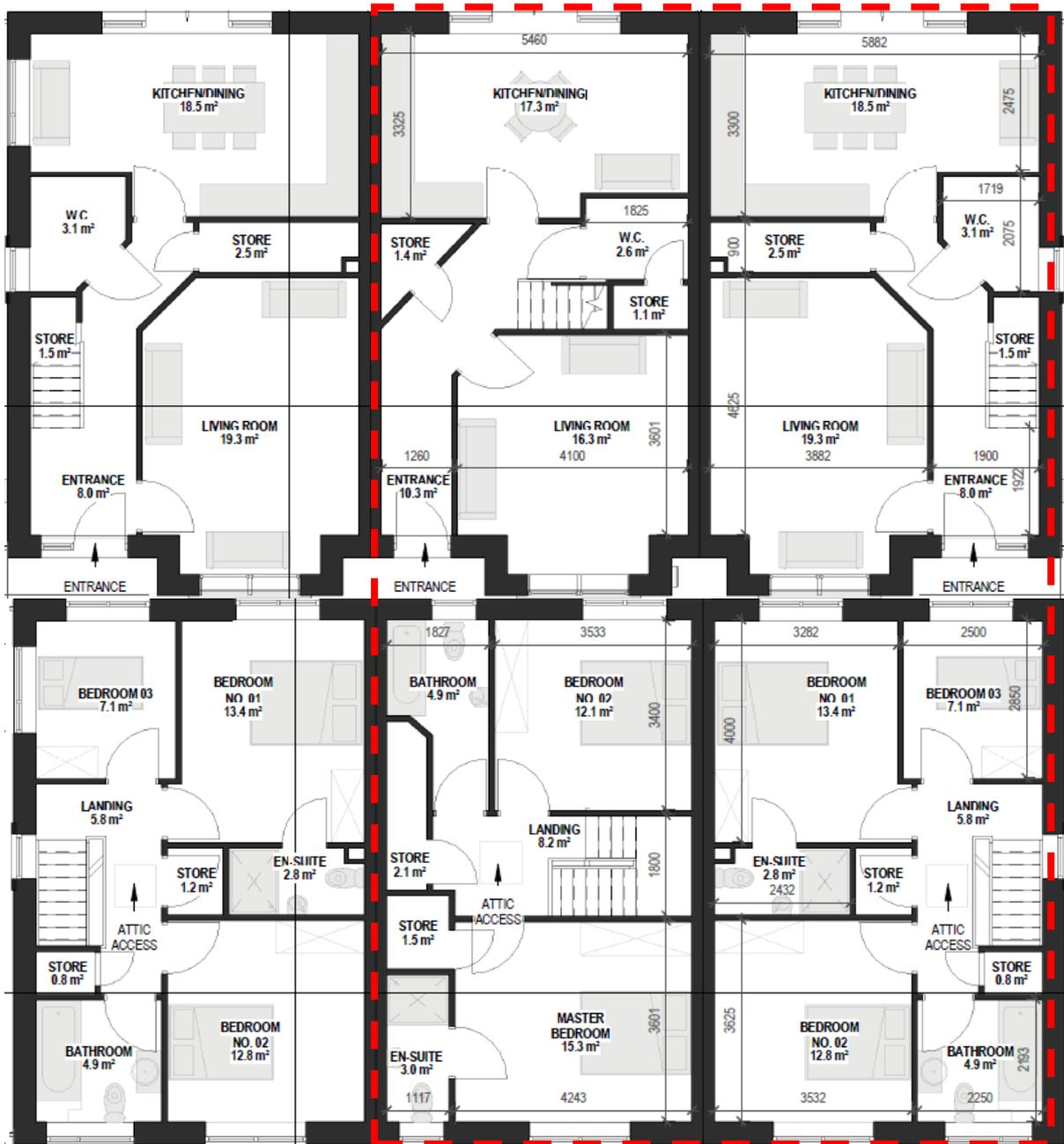
Figure 61.0 Typical ground floor plan of House Type 5.4 (top) and typical first floor plan of House Types 5.4 (bottom). The area within the red dashed line represents the ground and first floor plans for House Types 5.2-5.3.
