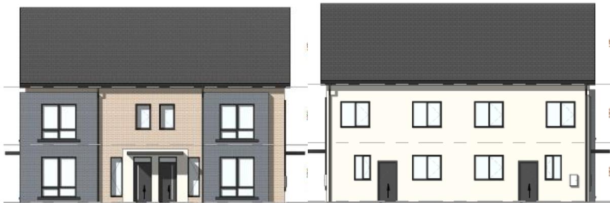
Figure 45.0 Front elevation (left) and rear elevation (right) of Maisonette buildings accommodating Maisonette Types 7.7-7.10.
