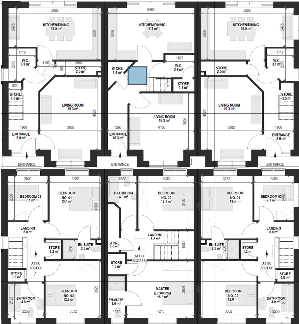
Figure 79.0 Typical ground floor plan of House Type 5.1 (top) and typical first floor plan of House Types 5.1 (bottom). The area within the red dashed line represents the ground and first floor plans for House Types 5.2 & 5.5.
