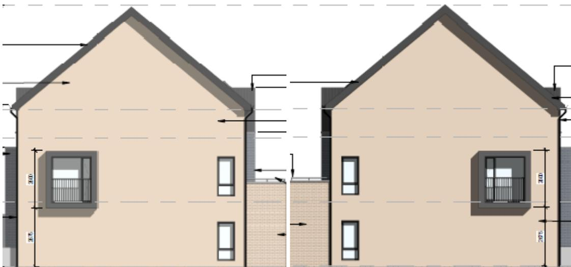
Figure 35.0 Side elevation No. 1 (left) and side elevation No. 2 (right) of the Apartment & Duplex Apartment Blocks.
