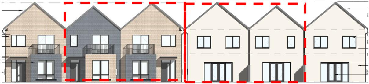
Figure 62.0 Front elevation of House Types 5.1 & 5.3 (left) and rear elevations of House Types 5.1 & 5.3 (right).
