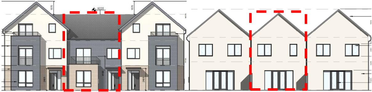
Figure 74.0 Front elevation of House Type 6.2 (left) and rear elevation of House Type 6.2 (right). The area within the red dashed lines represents the front and rear elevations of House Types 6.1 & 6.3.
