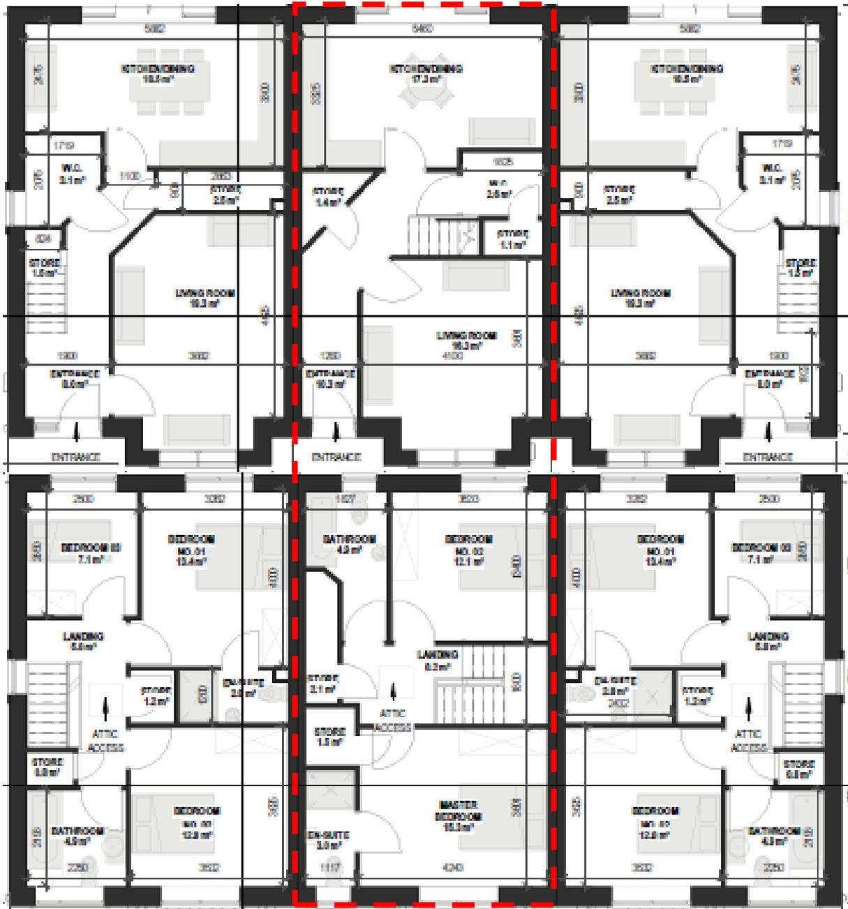
Figure 59.0 Typical ground floor plan of House Types 5.1 & 5.3 (top) and typical first floor plan of House Types 5.1 & 5.3 (bottom). The area within the red dashed line represents the ground and first floor plans for House Type 5.2.
