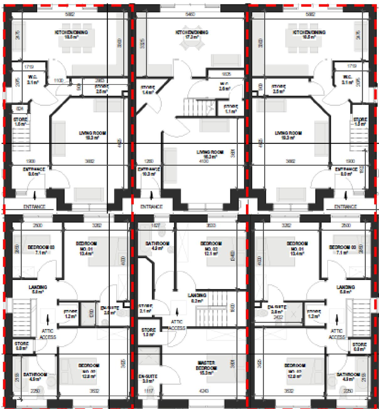
Figure 70.0 Typical ground floor plan of House Type 5.2 (top) and typical first floor plan of House Types 5.2 (bottom). The area within the red dashed lines represent the ground and first floor plans for House Types 5.1 & 5.3.
