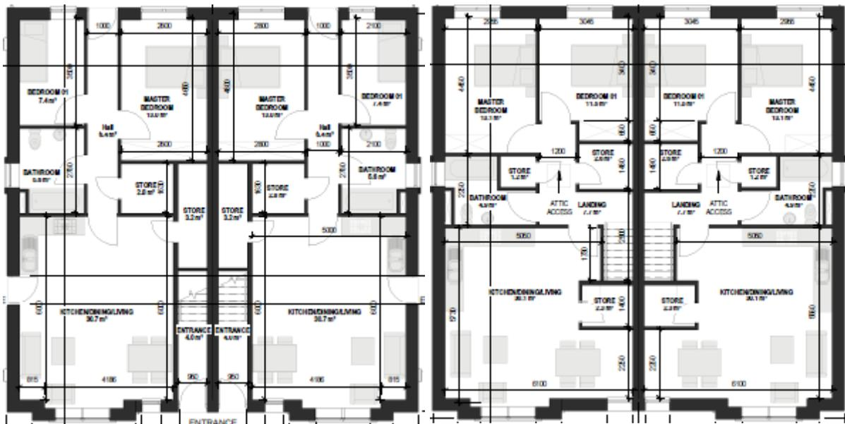
Figure 40.0 Ground floor level (left) and first floor level (right) of Maisonette buildings accommodating Maisonette Types 7.1-7.4.
