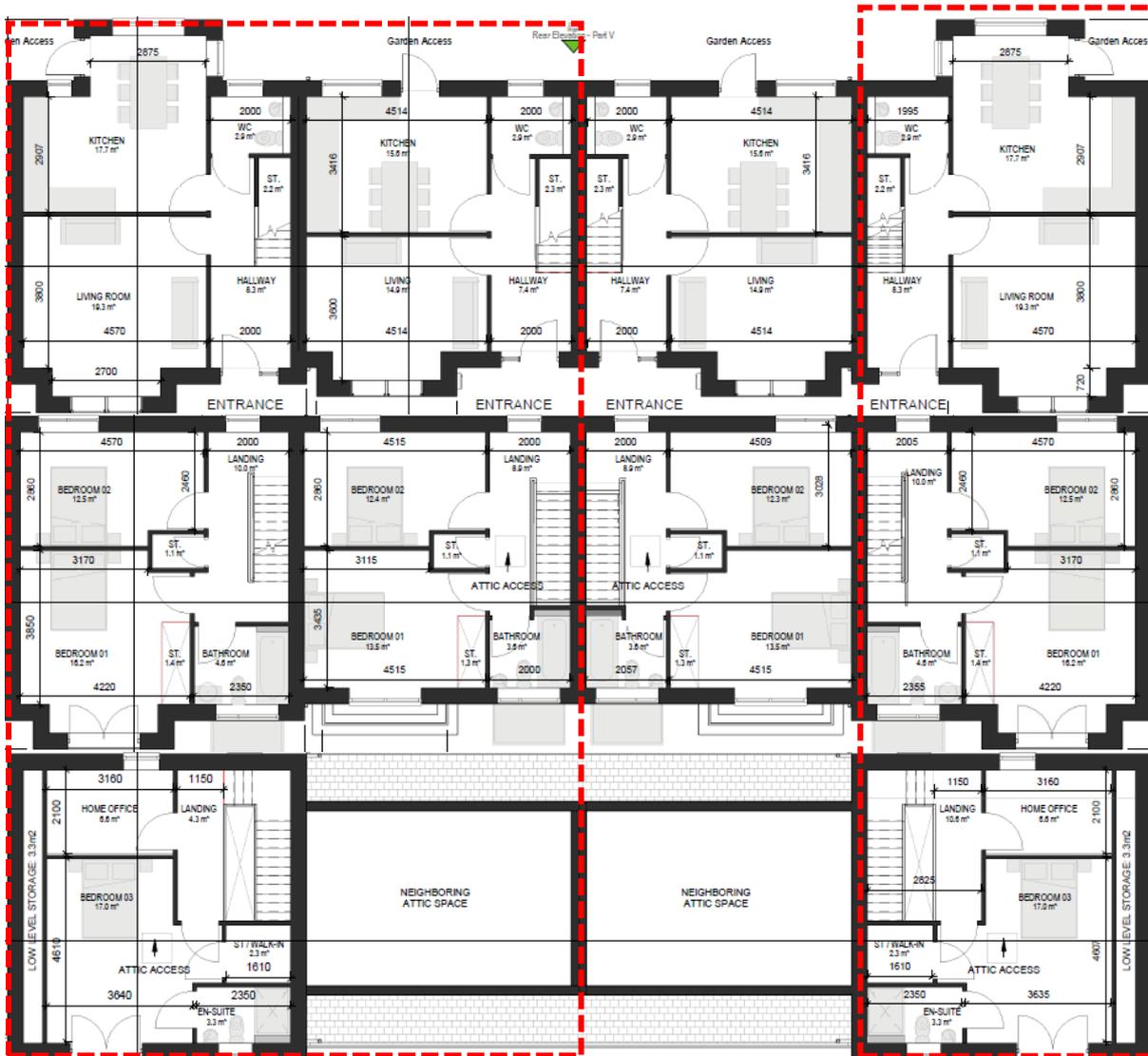
Figure 75.0 Typical ground floor plan of House Type 6.10 (top), typical first floor plan of House Type 6.10 (centre) and typical first floor plan of House Type 6.10 (bottom). The area within the red dashed line represents the ground, first and second floor plans of House Types 6.1-6.3.
