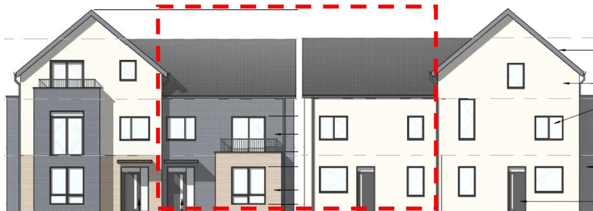
Figure 78.0 Front elevation of House Type 6.6 (left) and rear elevation of House Type 6.6 (right). The area within the red dashed lines represents the front and rear elevations of House Type 6.5.
