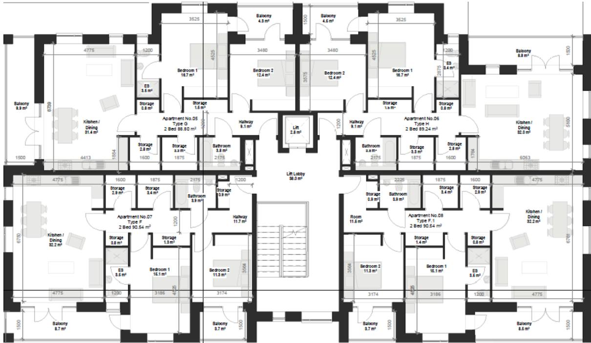
Figure 31.0 First and second floor plan for Apartment Block F. The ground floor plan of this block, which comprises the creche facility, is presented in Figure 81.0 of this report.
