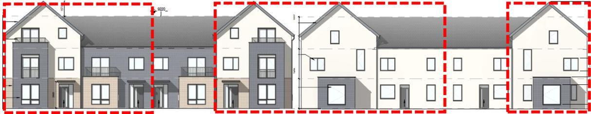
Figure 76.0 Front elevation of House Type 6.10 (left) and rear elevation of House Type 6.10 (right). The area within the red dashed lines represents the front and rear elevations of House Types 6.1-6.3.
