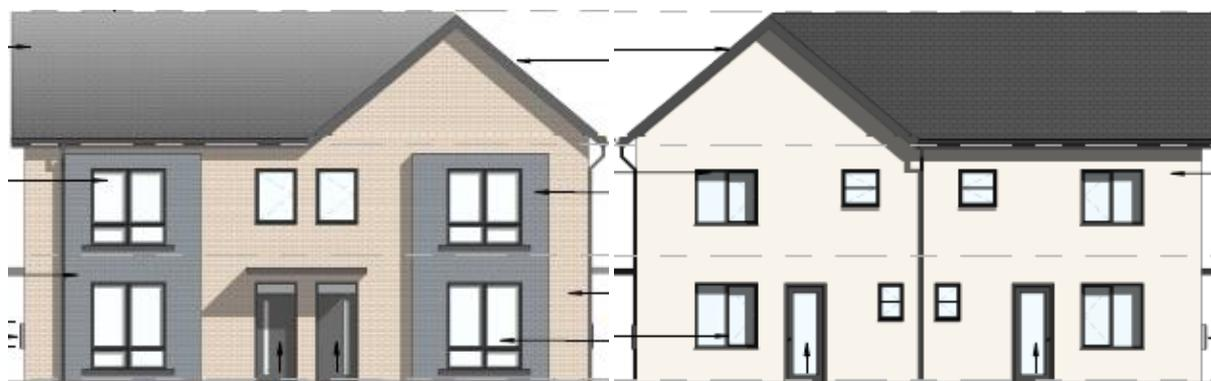
Figure 46.0 Front elevation (left) and rear elevation (right) of Maisonette buildings accommodating Maisonette Types 8.5-8.8.
