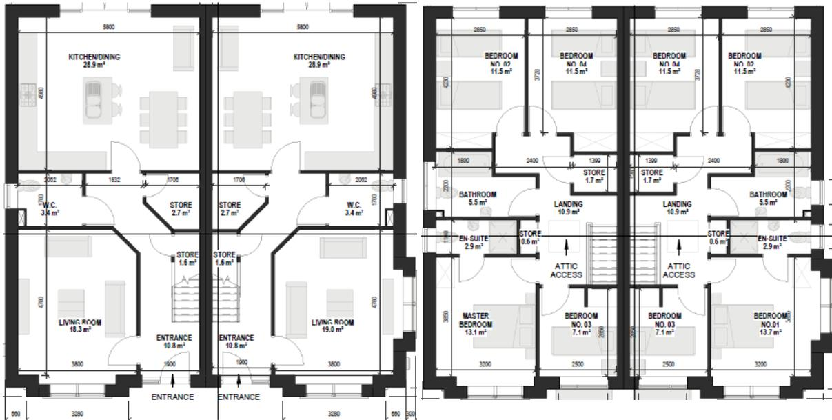
Figure 48.0 Typical ground floor plan of House Types 1.1-1.4 (left) and typical first floor plan House Types 1.1-1.4 (r).
