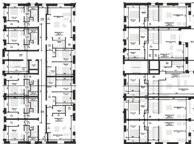
Figure 25.0 Second floor plan (left) of Apartment Block C and third floor plan (right) of Apartment Block C. As presented previously, only Building No. 2 of Apartment Block C rises above first floor level height.
