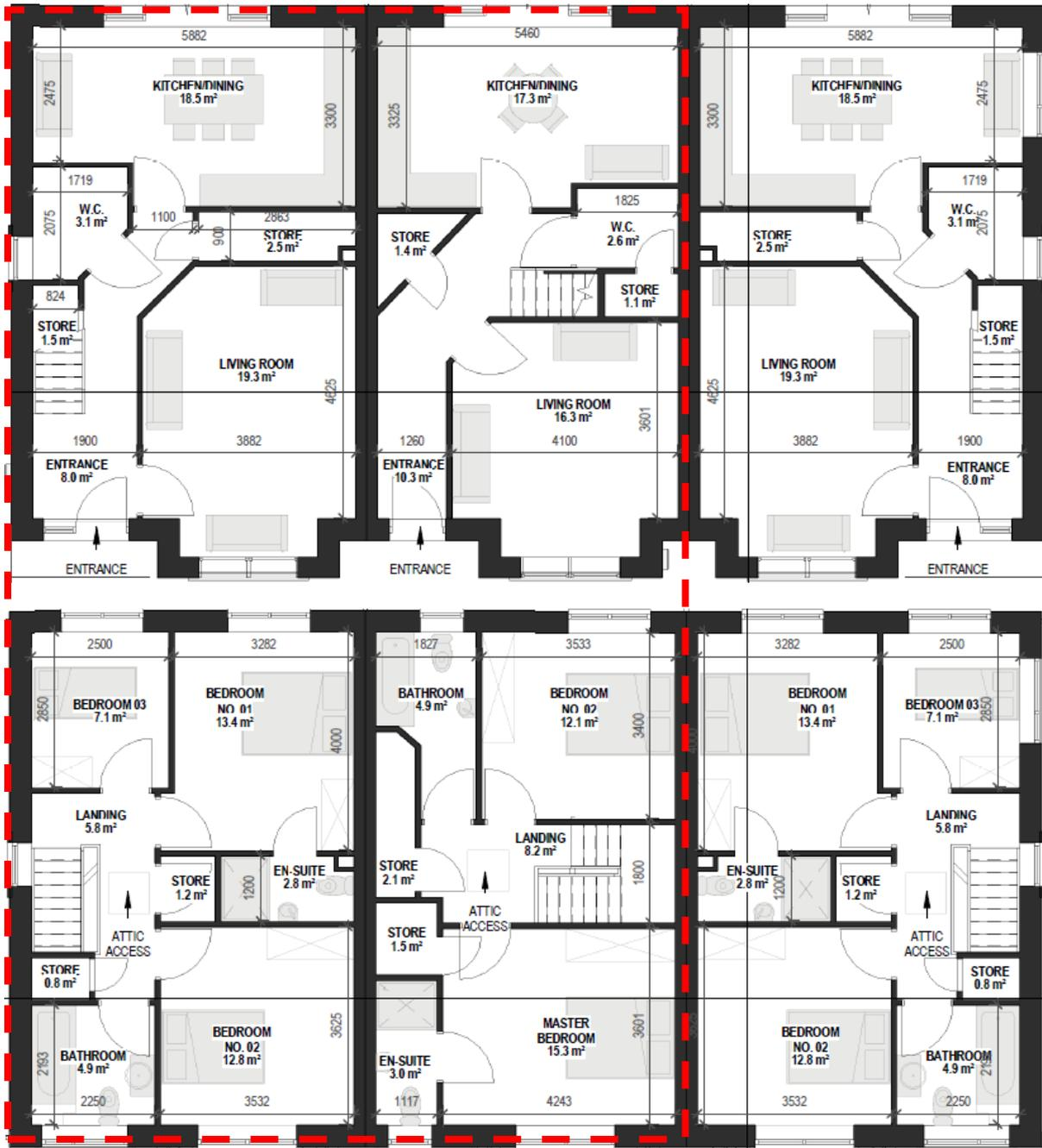
Figure 63.0 Typical ground floor plan of House Type 5.5 (top) and typical first floor plan of House Types 5.5 (bottom). The area within the red dashed line represents the ground and first floor plans for House Types 5.1-5.2.
