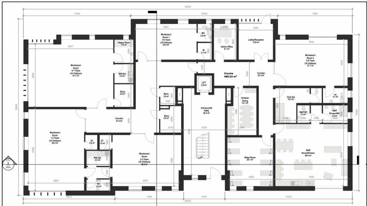
Figure 2.4 Proposed ground floor level of Block F illustrating layout of creche facility.
